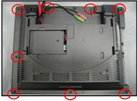
2. Un-install all screws on backhousing and remove back cover.
