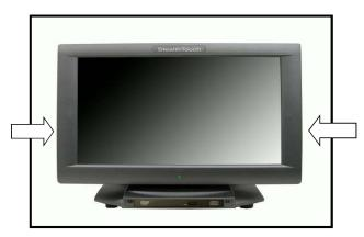
First unplug power cable from system. Then remove the system from the base by unscrew two screws on the side (see arrow). Then pull the system up and forward to remove it from the base stand.
