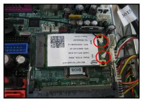
4. Plug antenna cable to wireless card.
