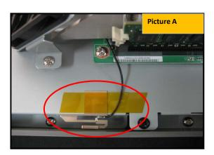
5. Tape other end of antenna cable to MB metal. Note: See picture A and B
